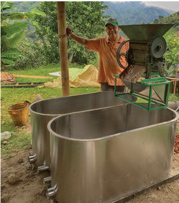
Coffee farmer Oscar Morales Ospina stands beside his new coffee washing tub. These washing tubs reduce the amount of water needed to wash coffee and help to treat the water so runoff does not contaminate the watershed
